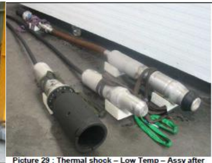
Picture 29 : Thermal shock - Low Temp - Assy after immersion
