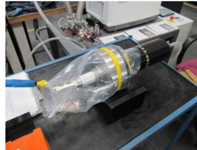
Picture 7: Helium leak test set-up.
