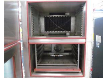
Picture 14: Thermal shock set up with location temperature sensor.
