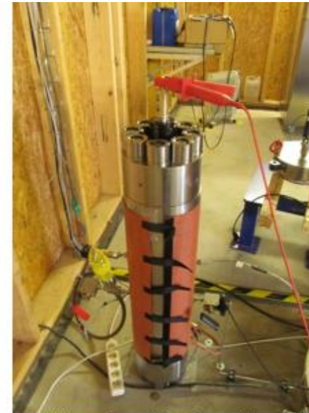
Picture 15: Pressure cycling set-up with clamp of megger connected.
