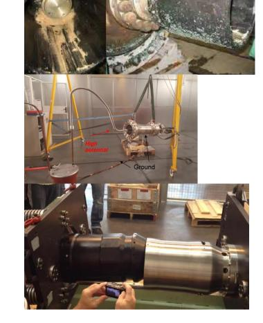
Penetrators have been submitted to 30 pressure tests at 1,5 x design pressure in both directions. Other specific tests for compressor penetrators have been done such as rapid gas decompression test.
